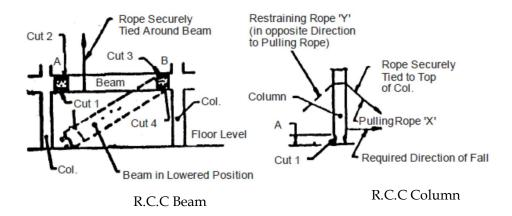
(c) Reinforced Concrete Walls Reinforced concrete walls should be cut into strips and demolished as for columns (shown in fig).
